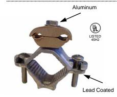
**#306A** - Bronze Large Perfection Pipe Clamp with clamp type cable fastener that swivels  $360^{\circ}$ . Fits 1 1/2" and 2" iron water pipes. (Max. 2 1/2" O.D.). Lower casting may be inverted to fit smaller diameter pipes and rods. Tinned to prevent corrosion. Wt. 1.04 lb. ea.  $\bigstar$
