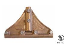
**#G181** - **Bronze Heavy Duty Three Way Connector** for 1/0 or 2/0 cables with bolt type cable connection used for "T" cable splice on roof and for connecting to counterpoise cable. Eliminates right angle connections. Connector has 8" of contact with horizontal cable and 4" of contact with vertical or branch conductor. Wt. 2.10 lb. ea.
