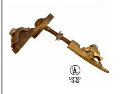
**#326** - **Bronze Feed Thru-Roof Connector** with ball and socket swivel for easy adjustment to roof pitch (no greater then 5/12 roof pitch). 3" length threaded stem with hex nut and washer, two wood screws and clamp type cable connector. Underside is recessed and can be filled with plastic roof cement to afford perfect weather tight seal. (Note: For longer stems use couplers and threaded studs that are found elsewhere in the catalog) Wt. 1.24 lb. ea. ★
