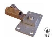
**#A183** - **Bimetal Bonding Plate** made of cast aluminum and bronze for connecting all standard copper cable through 2/0 to aluminum beams and other large structural aluminum metal bodies requiring 8 square inches of bonding surface as provided by the aluminum portion of this clamp. Connector has clamp type cable fastener. Wt. .60 lb. ea.  $\star$
