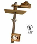
**#597X** - Bronze Right Angle Thru-Roof Connector consists of clamp type top cable connector, 4" square roof flashing plate, 1/2" x 8" threaded stem, hex nut and washer, and adjustable bottom clamp. Fits up to 6" roof thickness. If required for thicker roof, specify when ordering. Wt. 2.04 lb. ea.
