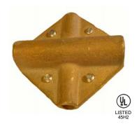
**#G95** - **Bronze Large Heavy Duty Cross Run Connector** with hex-head screws. Measures 4" x 4" and used for bonding standard cables through 2/0 to 1/2", 5/8", or 3/4" dia. ground rods at right angles. When ordering, please specify size of ground rod and cable. Wt. 1.22 lb. ea.
